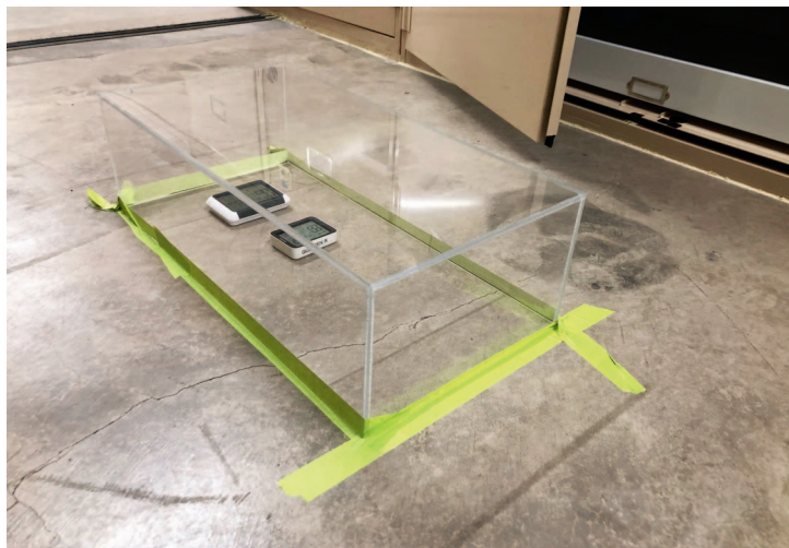
Figure 8. Improvised sealed enclosure to measure humidity emanating from the concrete floor of the collections building, September 2020. Note the strip of silicone seal along the base of the cabinets.
