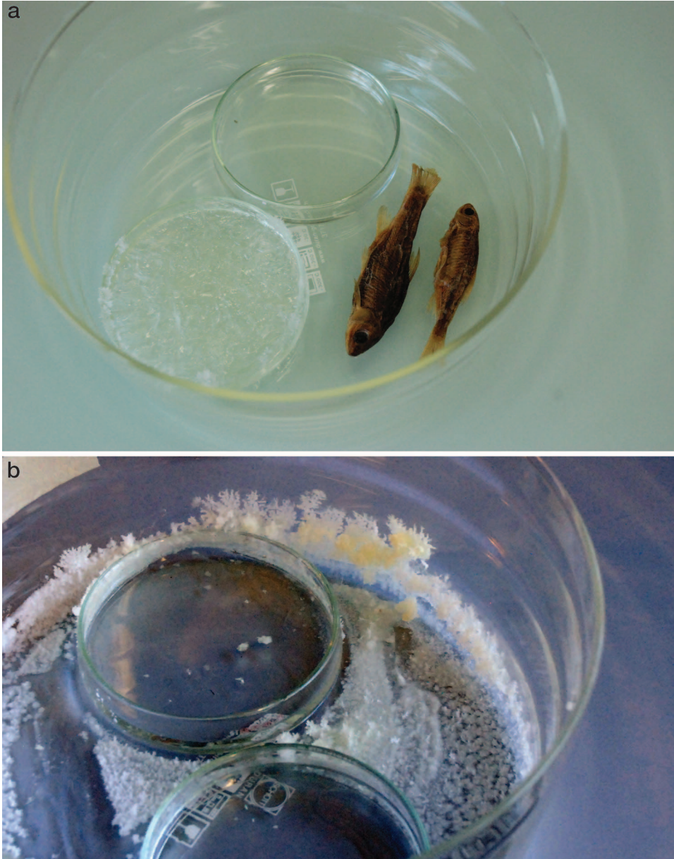
Figure 1. (a) Benzoic acid crystallization on Petri dishes after 24 hours of treatment. (b) Extreme benzoic acid crystallization after 4 days of exposure in a test of growth speed without specimens (© NMBE, F. Neisskenwirth).
